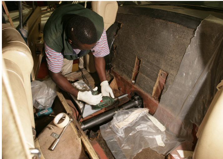
Above: Quickfit team secures new anchors for seatbelts beneath rear bench. Main: fabric for belts chosen to match Rapide's cream leather
