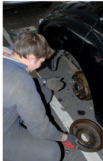
Drum check revealed leaking cylinder
