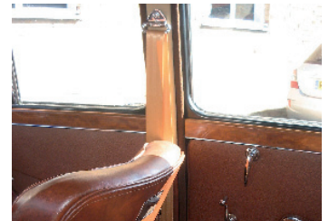
Neatly fitted B-post inertia-reel bracket
