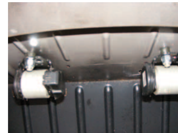
Inertia reels are concealed under the rear parcel shelf.
