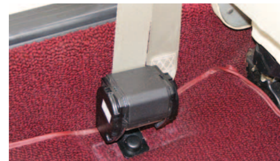
The front set up is much neater than the original ever was, with the smaller reels being bolted to a concealed bracket on the floor. The impression of the original and much larger Britax reels can be seen from the indentation on the carpet.
