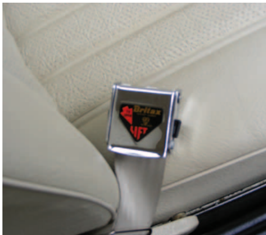
The original Britax buckles were used with new webbing in the front.
