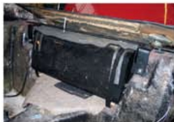
Neat brackets anchor harnesses to chassis
