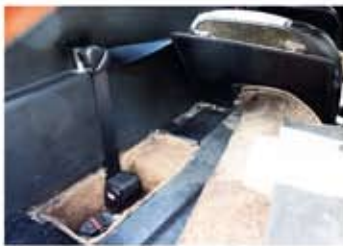
...and secures inertia reel beneath floor
