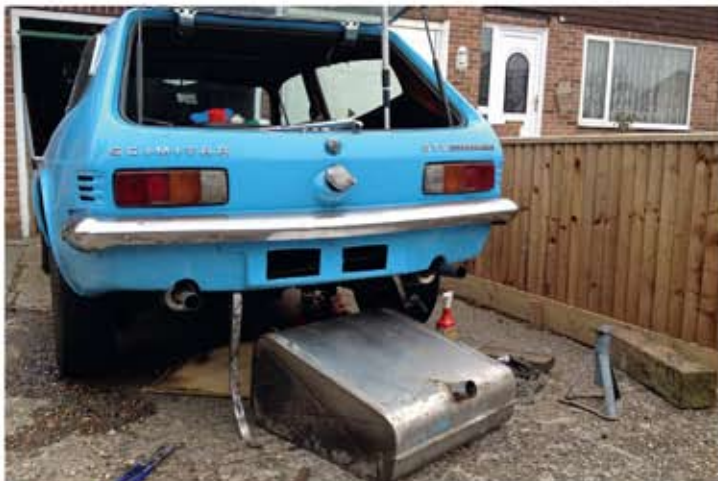
Broken strap hanging down and tank finally on the floor. And yes, that is fuel everywhere
