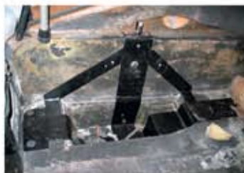
Ingenious bracket fixes to body mounts...
