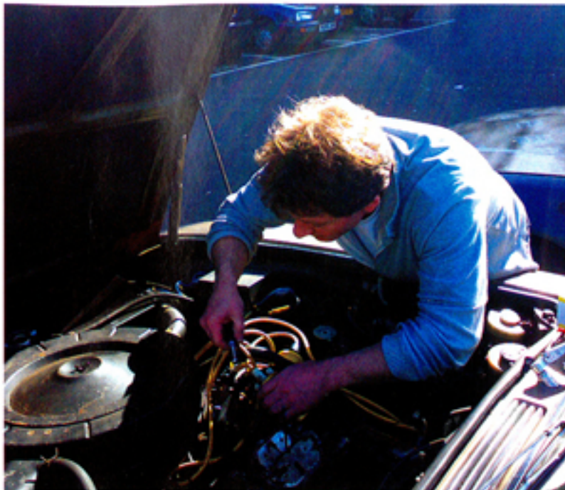
Pricy Mopar coil has smoothed out power delivery from the Jensen's Chrysler V8
