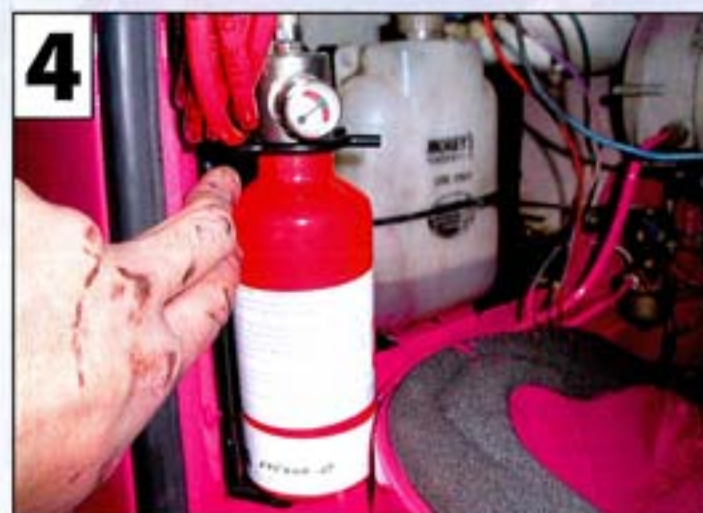
As shown in Fig 3 clip the bottle and flexi hose combined, to the bottle clamp you have just screwed on. Now this is one of the things you must be aware of, make sure you can see the bottle gauge, so face the gauge where you can see it at a glance so you can check the condition of the extinguisher bottle before you start to tie on the flexi hose. (Fig 4)
