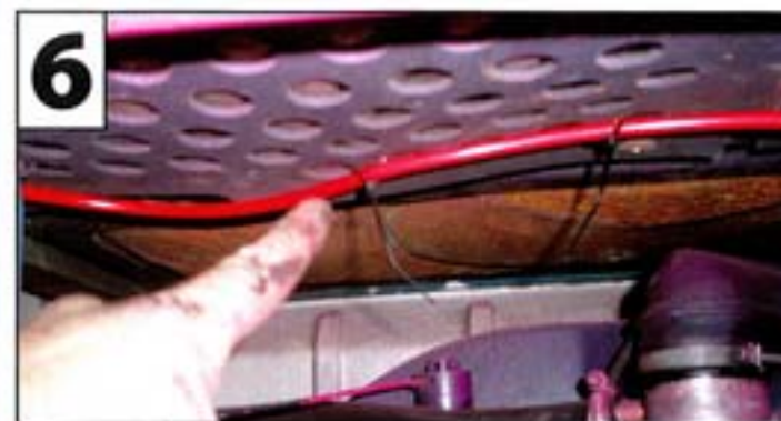
Then, as in Fig 6, if you have a rear engine like my 1972 Westy, tie the flexi hose with the ties provided to the cardboard grid above the engine, cutting off the ends of the ties when you have fixed them for neatness.
