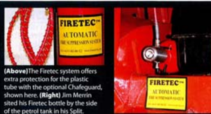
Carefully unravel the flexi hose without twisting it as you don't want to fracture it! (Fig 5).
