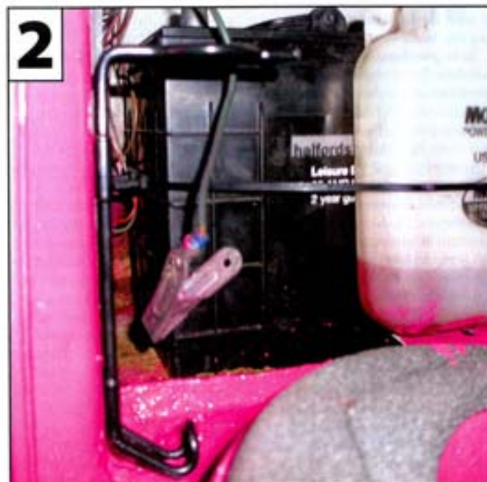
The first thing you need to do is decide where you are going to site the extinguisher bottle. If, like me, you have a big leisure battery in the spare battery compartment, then I found the best place to fit this size bottle was on the post just inside the engine bay as shown in (fig 2). Drill two holes, and using the screws provided with the kit, screw the bracket to the post as shown.
