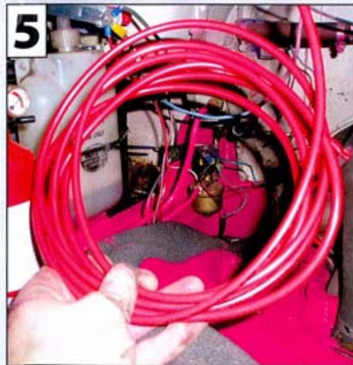
Carefully unravel the flexi hose without twisting it as you don't want to fracture it! (Fig 5).
